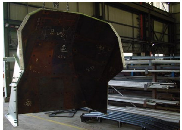
Fabricated mild steel galvanised chute supplied with studded wear plate set.
